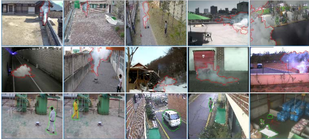
Fig. 9. Smoke detection results Red boundaries are detected smoke regions; green boundaries non-smoke moving objects
