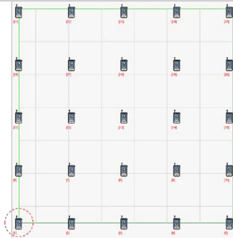
Fig. 8. An example for a given network, 25 IoT-sensor nodes for single-zone
