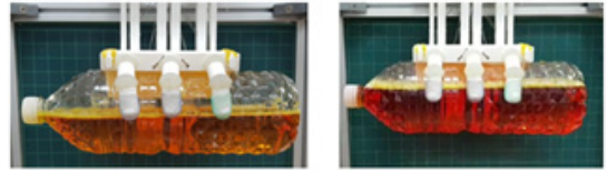
Fig. 11. Gripping test at 1000 g, and 1800 g
