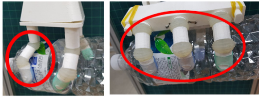
Fig. 9. Gripping shape comparison between the previous soft gripper and the proposed soft robotic hand
