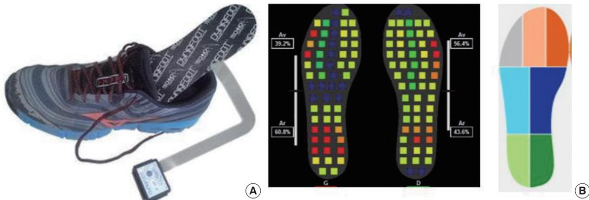
**Figure 2.** Dynamic pressure mapping system. (A) Insole sensor and module, (B) Measurement areas of pressure.
