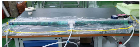
Fig. 11. Infusion process of CFRP TIE ROD
