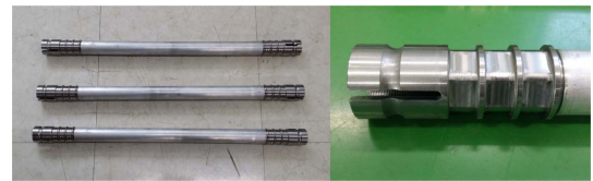
Fig. 2. Core shape of CFRP TIE ROD
