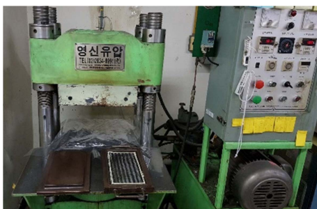
Fig. 2. Hot press forming equipment
