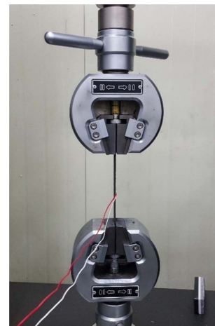
Fig. 3. Tensile test procedure of braided carbon/epoxy composites
