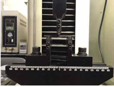
Fig. 4. Flexural test procedure of braided carbon/epoxy composites
