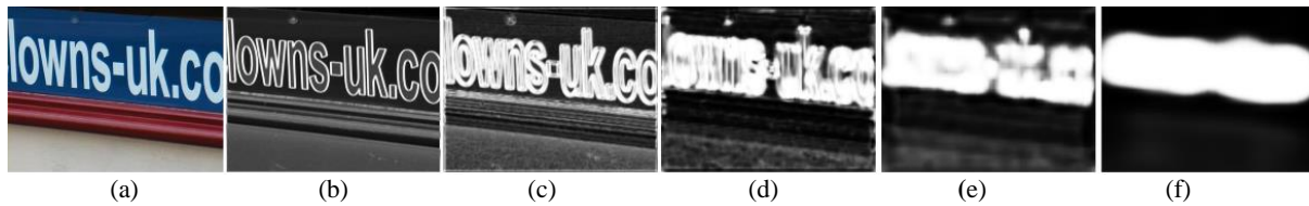
Fig. 4. Example of Feature-map Generation from the Usage of the Supervised Fully Convolutional Network (FCN). (a) Input image, (b)-(e) feature maps from stages 1-4, and (f) feature maps for stage 5 and the final salient map
