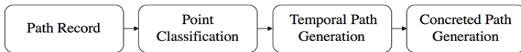
Fig. 1. Generation a path using the user’s records consists of four stages: Path Record, Point Classification, Temporal Path Generation, and Concreted Path Generation.
