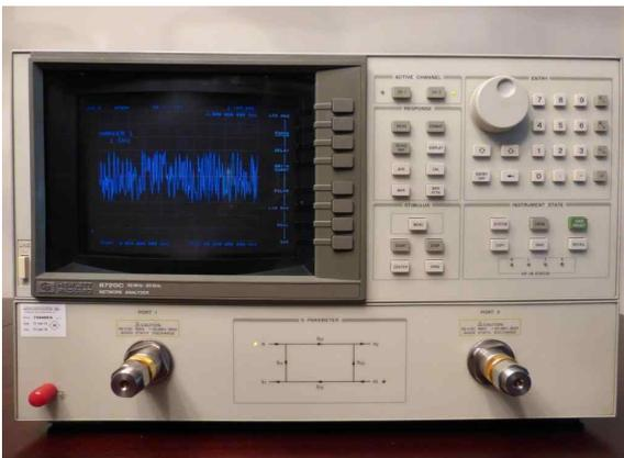
Fig. 7 Network analyzer
