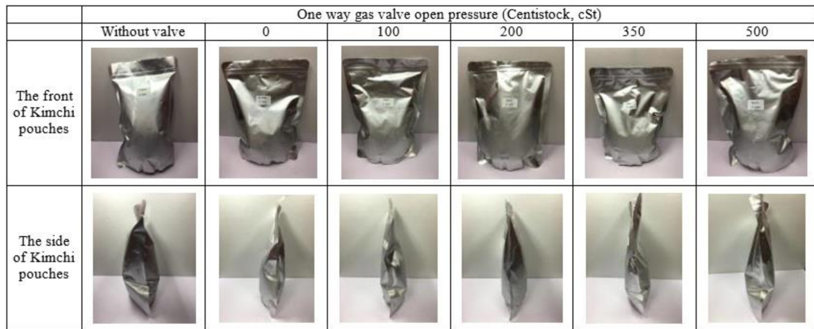
Fig. 3. Differences in volume expansion of Kimchi packages with and without the one-way valve at different open pressure levels at 4 weeks.
