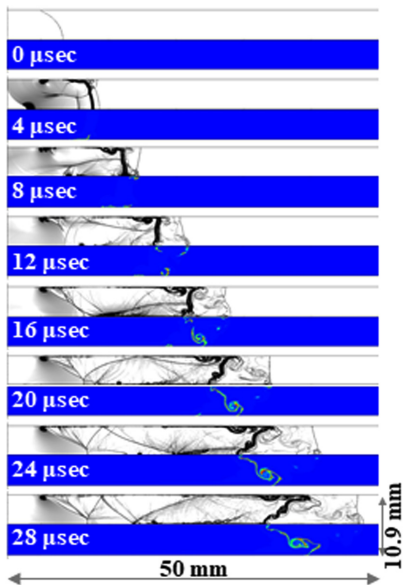
Fig. 8. Initial flow development inside 10.9 mm tube ; Schlieren and OH radical.
