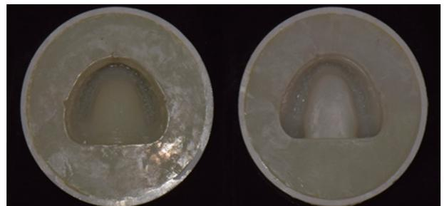
Fig. 3. Silicone mold for wax denture.
