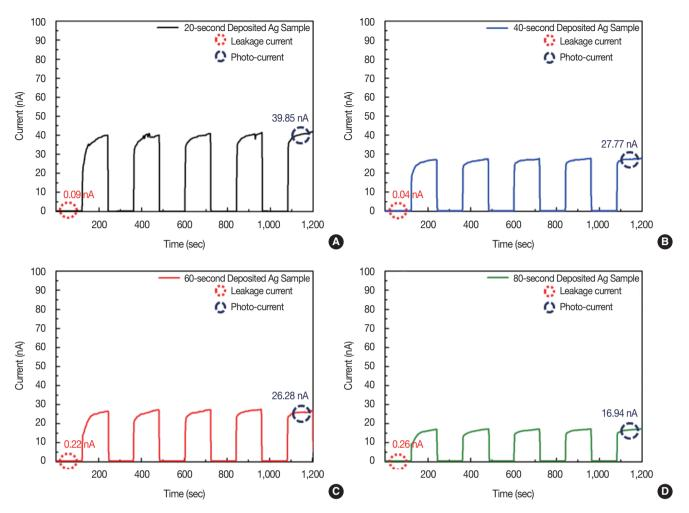
Fig. 4. Leakage current and photo-current under 254-nm UV irradiation for (A) 20-, (B) 40-, (C) 60-, and (D) 80-second deposited thin-film Ag electrodes on CVD diamond.
