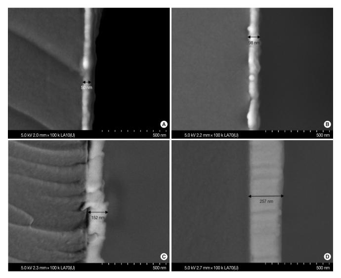
Fig. 2. SEM images of cross-sectional thickness of (A) 20-, (B) 40-, (C) 60-, and (D) 80-second deposited thin-film Ag electrodes on the glass substrate.
