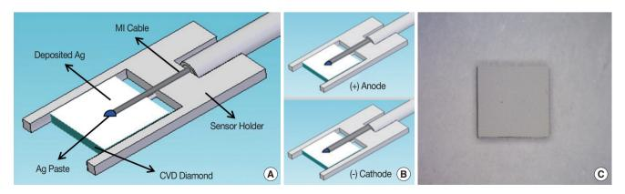
Fig. 1. Diagram of MI cable connection to deposited thin-film Ag electrode on CVD diamond (A); cathode and anode side of deposited thinfilm Ag electrode (B); picture of deposited thin-film Ag electrode on CVD Diamond (C).
