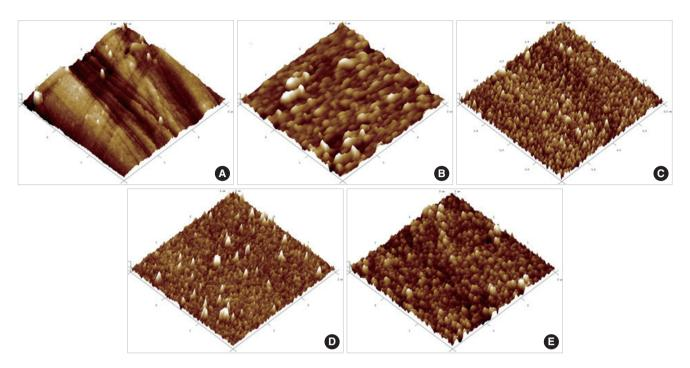
Fig. 3. 3D AFM images of (A) the surface of the bare diamond substrate, and the (B) 20-, (C) 40-, (D) 60-, and (E) 80-second deposited thinfilm Ag electrodes on the glass substrate.
