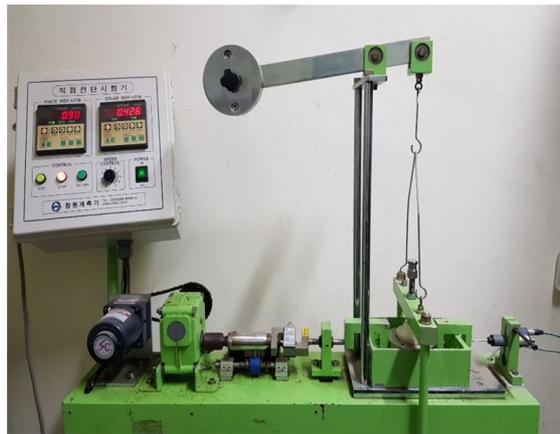
Fig. 3. Direct shear tester
