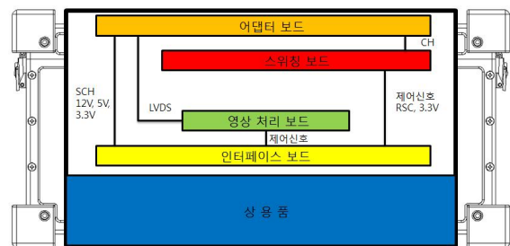
Fig. 3. Block diagram on TAS-815K ATE
