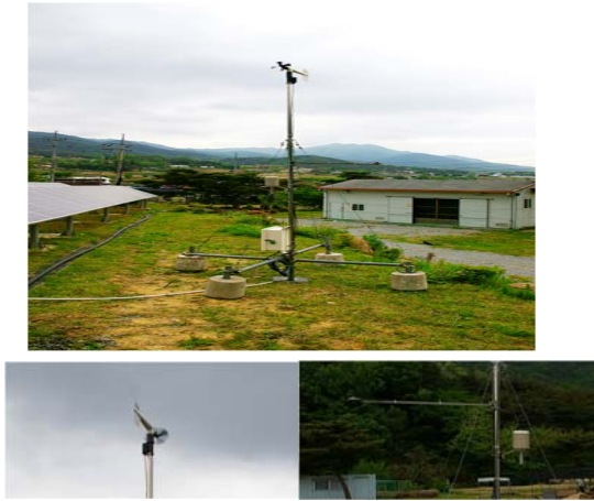
Fig. 1. Photograph of field weather observation system established at New Solar Power Plant Cooperation.
