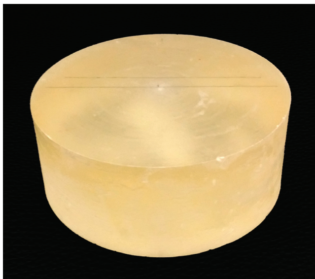
Fig. 1. The acrylic phantom used in this study. A metal sample is positioned in the phantom.
