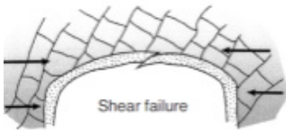
(g) Shear failure of stiff/brittle membranes
