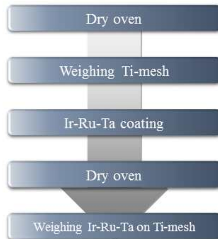
Fig. 2. Manufacturing step of Ir-Ru-Ta/Ti-mesh using brush coating.
