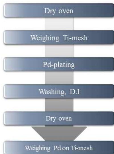
Fig. 1. Manufacturing step of palladium electroless plating.
