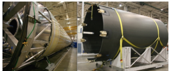
Fig. 3 Falcon 9 lightweight structure, (left) aluminum-lithium (right) carbon-fiber composite[5].
