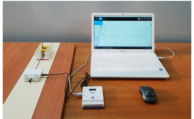
Fig. 5 Measuring the force of kinetic friction by using the force sensor equipment
