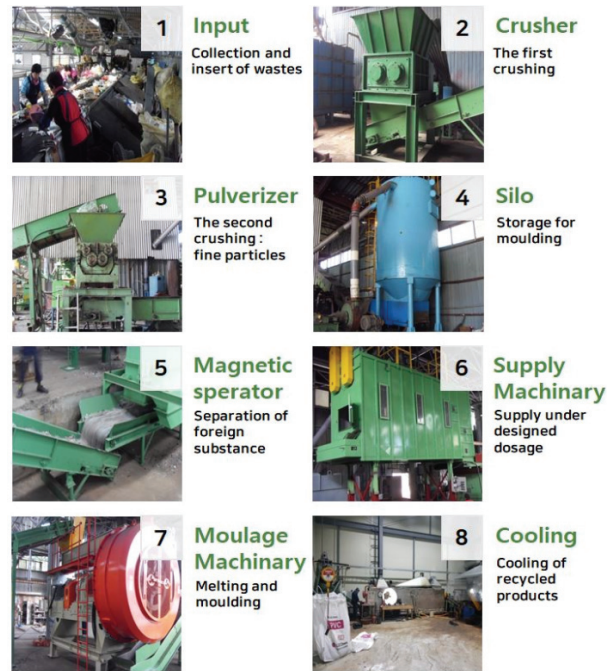
Fig. 1. Typical process for producing molding materials recycled using film packaging wastes
