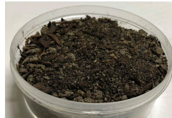
Fig. 7. Manufactured artificial lightweight soil
