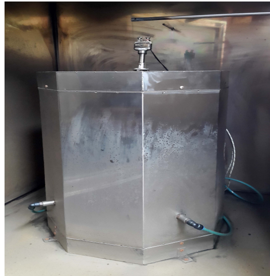
Fig. 1. Combustion furnace for thermal pyrolysis of wood.
