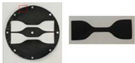
Fig. 3. Manufactured test specimen.
