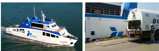
Fig. 1. Mobile LNG Refueling by Tank-lorry[1]
