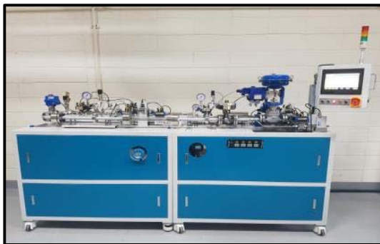
Fig. 7. Excess Flow Valve performance test facility in KGS.
