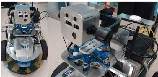
Fig. 6. The multi-modal sensor module mounted on robot platform.
