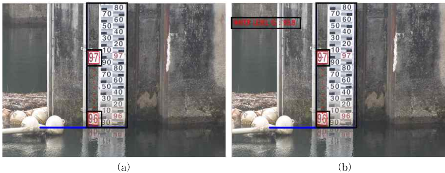
Fig. 8. Water level detection, (a) Virtual scale drawn according to water scale format, (b) The scale check with the water level line and display the current level.
