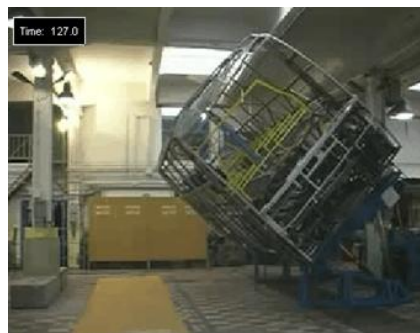
Fig. 2 Bus rollover experiment ( https://www.youtube.com/watch?v=KYm-L5i8_5o )
