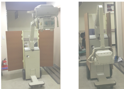
Fig. 4. Mobile X-ray Generator Installed with a assembled Shield.
