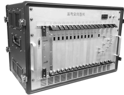
(b) 제작된 표적모의장치 (b) Manufactured target simulation equipment
