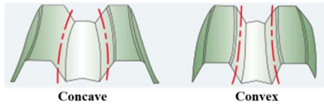
Fig. 4. Curvic coupling teeth (Concave and Convex).
