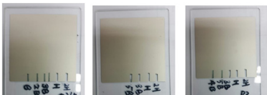
Ag paste(1) Ag paste(2) Ag paste(3) Fig. 9 Pencil hardness results of Ag paste
