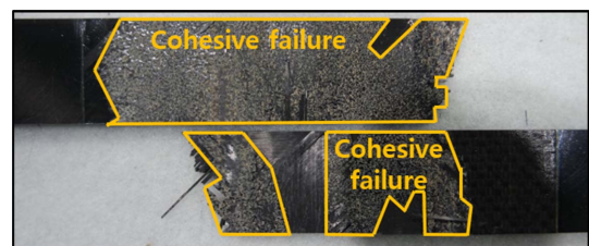
Fig. 10. Typical failure mode (0 atm, heat-blanket)
