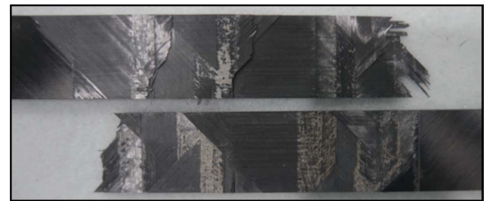
Fig. 14. Typical failure mode (1 atm, heat-blanket)
