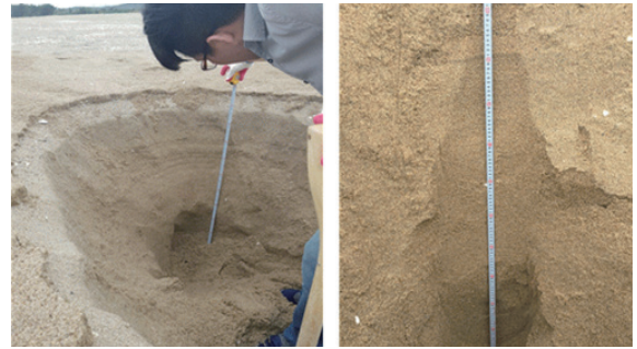
Fig. 2. Sampling up to 100 cm with every 20 cm spacing in estuary sand sediments area from the Namdae-cheon stream
