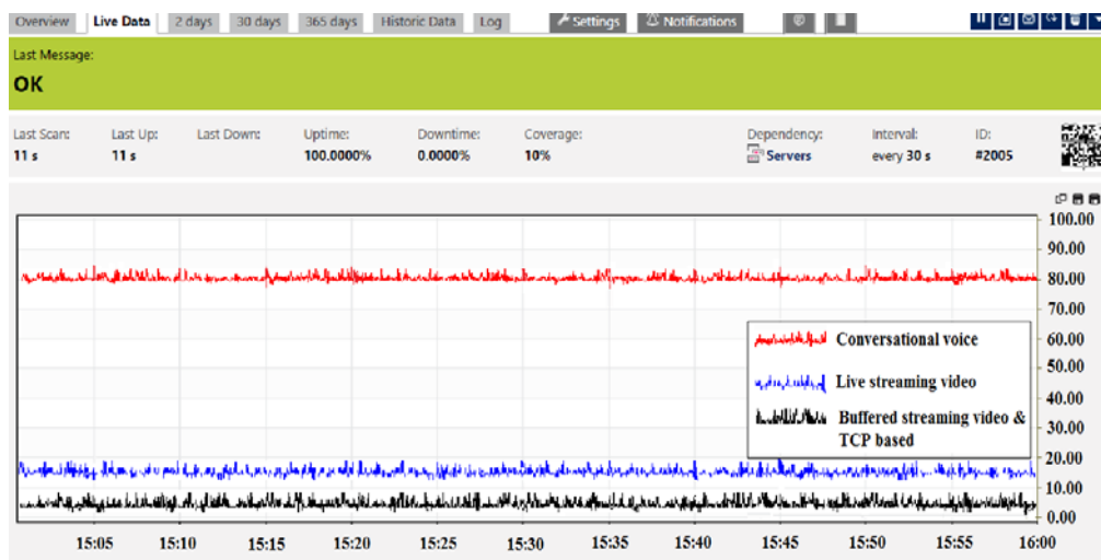
Fig. 17. Time trace of process utilization ratio for conversational voice, live streaming video and buffered streaming video and TCP based traffic
