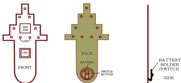
Figure 2. Smart Wappen Device Structure and System
