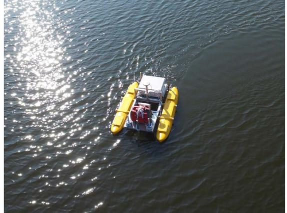
Fig. 8. USV used in the experiment
