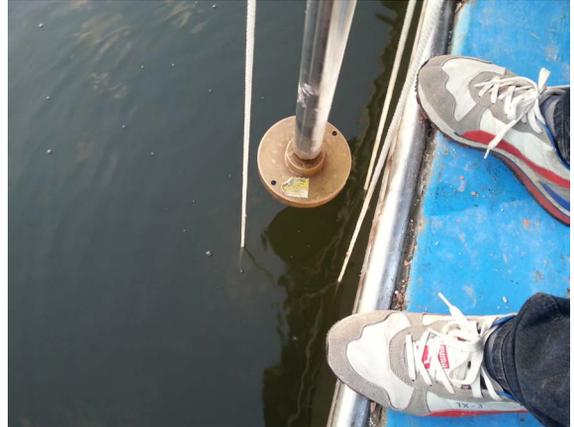
Fig. 11. Bar check of single beam echosounder
