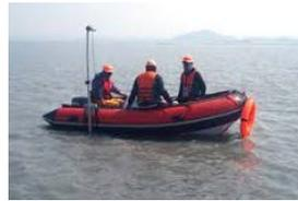
**Fig. 1. Measuring of water depth using rubber boat(Geosurvey.co.kr)**
