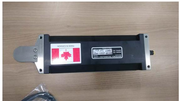
Fig. 6. Multi beam echosounder
