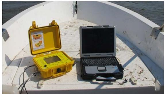
Fig. 5. Single beam echosounder
