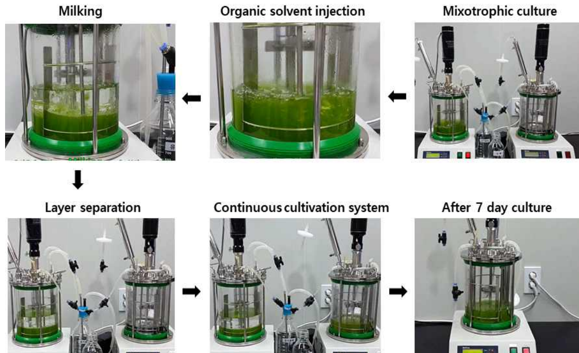
Figure 3. Flow diagram of continuous culture system through milking of C. protothecoides grown in culture during 7 days
