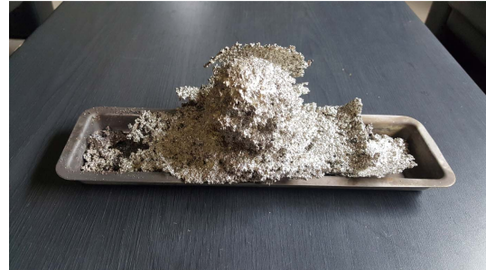
Fig. 3. The crude Tin obtained by gas reduction of waste tin oxide.
