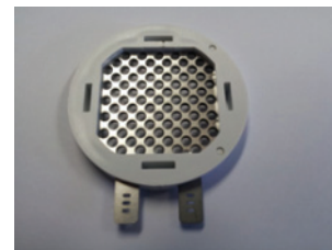
Fig. 2. Electrode of dielectric discharge.
