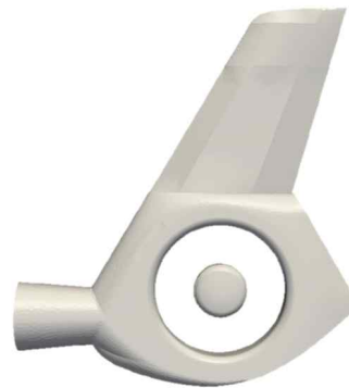
Fig. 2. Geometry of ducted fan tail rotor for validation
