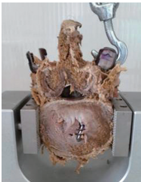
Fig. 2. The left pedicles of the 5th lumbar vertebrae were used for trans-endplate screw fixation penetrating the upper end plate, 2 mm distal to the pedicle entrance the lumbar pedicle screw was introduced 30° cranially to penetrate the superolateral and anterior aspect of the end plate. The right sides of the 5th lumbar vertebrae were used for anatomical trans-pedicular screw fixation through the body parallel to the end plate.
