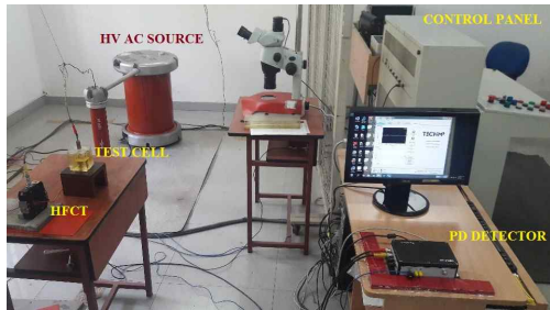
Fig. 4. (a) Schematic diagram of the laboratory PD measuring setup (b) Corresponding photograph of lab facility
