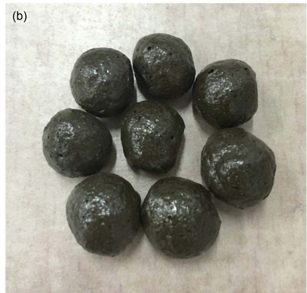
Fig. 7. Images of ultra-light ceramsite (a) SEM and (b) appearance.
