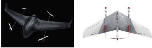
Fig 6. Fixed wing compound drone example [7]
