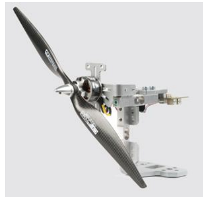
Fig 14. Thrust tester (RC Benchmark 1580) [8]
