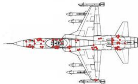
Fig 2. Defect distribution of F-5 EWIS
