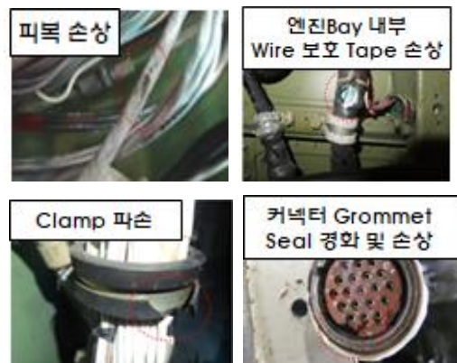
Fig 3. Defects type of aging aircraft EWIS
