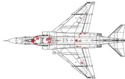
Fig 1. Defect distribution of F-4 EWIS
