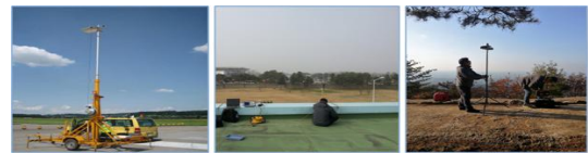
Fig 1. Typical ground inspection method for NAVAID
