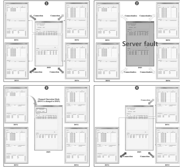
Fig 5. Non-disruptive server process in DSM
